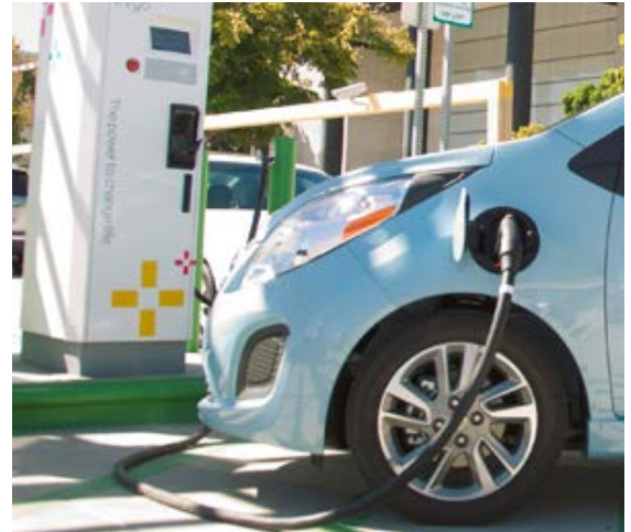
Figure 1.5: DC Fast Charging EVSE and SAE / CHAdeMO Connectors
