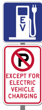
Figure 3.9 Recommended Signage for EV Charging
